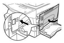
Ensure that the power switch of the machine is in the OFF position. Plug the other end of the power cord into the nearest outlet.
